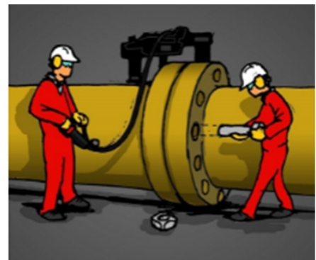
Powermaster flange alignment method
