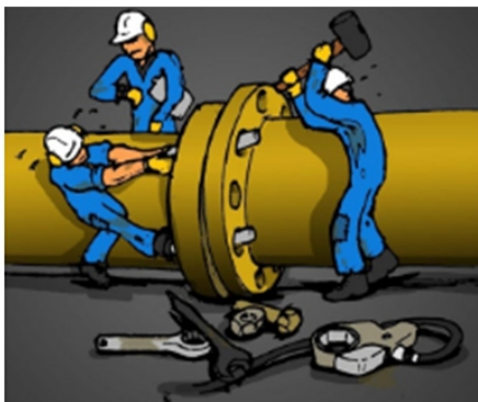
Traditional flange alignment method
