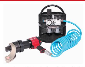
It is used to regulate the air pressure and properly lubricate the air motor for ultimate life. The Regulator regulates the inlet air pressure and controls the output torque of pneumatic torque wrench. All pneumatic tools must be used with FRL Unit. It is strongly advised not to exceed the maximum operating pressure as specified in the individual tool certificate.
