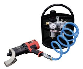
It is used to regulate the air pressure and properly lubricate the air motor for ultimate life. The Regulator regulates the inlet air pressure and controls the output torque of pneumatic torque wrench. All pneumatic tools must be used with FRL Unit. It is strongly advised not to exceed the maximum operating pressure as specified in the individual tool certificate.
