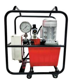
The PM-EH-1500 Electric motor with gear pump are designed to provide optimal service with bolt tensioner or hydraulic tools single-acting. Equipped with remote control with 5 m. cable for an easy use, 5 Ltr. tank, electromagnetic level and protective framework. It is an ideal tool under all job conditions.
