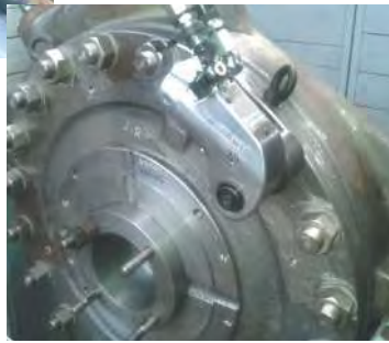
◀ PSD-3 Bolt tightening of Centrifugal pump casing
