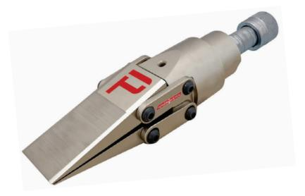
The Hydraulic spreader HSW-14, an efficient and versatile solution ideal for pipe and flange repair, as well as tasks such as removing elbows, gasket and metal seal replacement on couplers, and heavy equipment maintenance. Capable of delivering up to 15 metric tons of force, this lightweight (8.2 lbs. / 3.7 kg) spreader offers an ergonomic design, ensuring ease of use and optimal performance across a wide range of applications.
