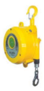
These balancers are provisioned with wire arrest mechanism, which locks the drum pulley in case of tool disengagement. These balancers are available for capacity from 9 - 70 Kg. & have all the feature of SWF balancers as well. These balancers are primarily used with welding guns and applications where chances of wire slitting or tool disengagement due to accidental failure are higher.
