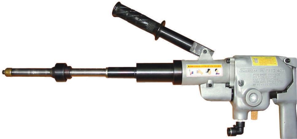
The design of these tube cutter are such that they cut ferrous and non ferrous tubes quickly and effortlessly. A constant feed rate of the cutting bit is achieved by combining high torque motors with our lever assist unit. It results in higher productivity and an extended life of the cutter.
